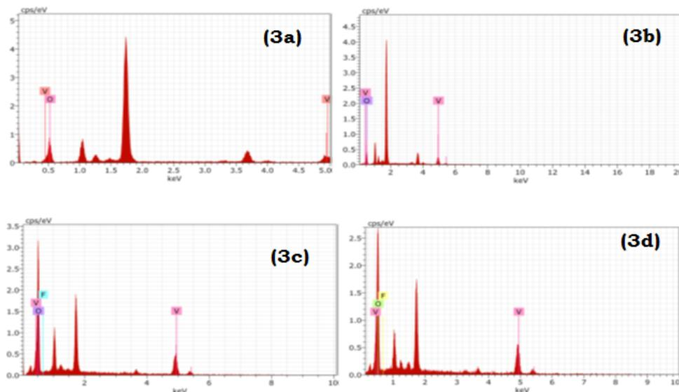
**Figs. 3a-d:** Compositional analysis of vanadium oxide thin films prepared by  $S_1$ ,  $S_2$ ,  $S_3$  and  $S_4$  solution.
