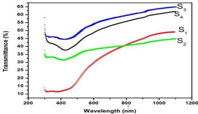
**Fig 4: Transmittance spectra of vanadium oxide thin films prepared by S<sub>1</sub>, S<sub>2</sub>, S<sub>3</sub> and S<sub>4</sub> solutions.**
