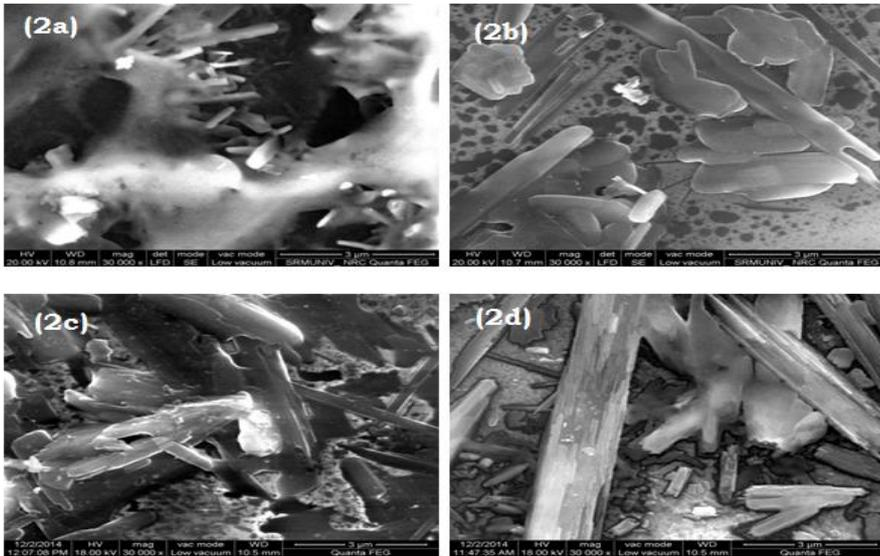
**Figs. 2a-d:**SEM image of vanadium oxide thin films prepared by  $S_1$ ,  $S_2$ ,  $S_3$  and  $S_4$  solution.
