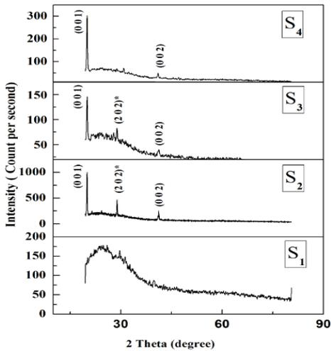
**Fig.1: X-ray pattern of vanadium oxide thin films deposited at 400°C from S<sub>1</sub>, S<sub>2</sub>, S<sub>3</sub> and S<sub>4</sub> solutions.**
