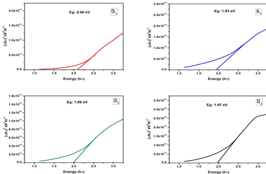
**Fig 5: Band gap of vanadium oxide thin films prepared from S<sub>1</sub>, S<sub>2</sub>, S<sub>3</sub> and S<sub>4</sub> solutions.**
